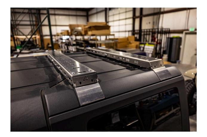
Starting with the front rails, place the connector plates on the inside as shown and install the eight M6x14mm bolts and M6 nylon lock nuts. Also install the four M6 bolts and nuts at the four corners of the rail as shown.
