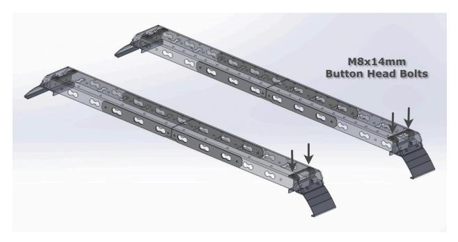
Once you have placed both rails on the roof and are satisfied that they are positioned correctly you may begin tightening according to the steps shown below.
