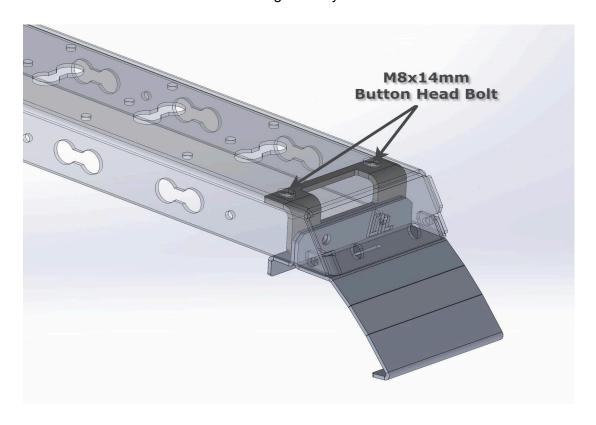
At the rear of the hard top, there are two  $4-\frac{1}{2}$ ' long slots on each side. Place the assembled bracket outer clamp edge into the slot and over the top edge of the roof.
