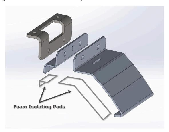
Loosely assemble the Mounting bracket, clamp and nut plate as shown using the M8x20mm button head bolts.
