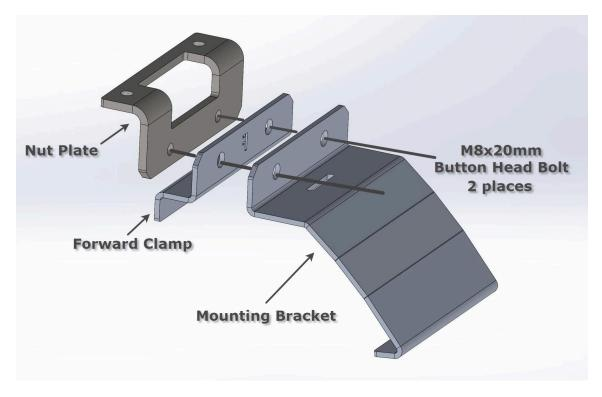
At one end of the rail, loosely assemble the corresponding clamp using the M8x14mm button head bolts. NOTE: Your front rail will be longer than your rear rail.
