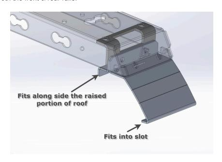
Next place the corresponding rail and assembled clamp on the opposite side and over the opposing clamp. Install the two M8x14mm button head bolts in the top two holes
